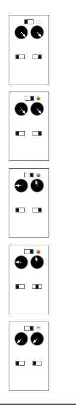
BEFORE SWITCHING ON, set both the control knobs to Maximum, Track1 direction to REV and Track2 direction to FWD.
