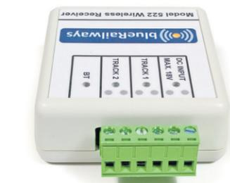
There are only six terminals at the rear of the Model 522 receiver unit: one for a power supply, usually from a low-cost wall socket transformer. The other two pairs are for track 1 and track 2 respectively.
