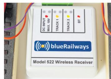
There are indicator LEDs fitted to the compact wireless receiver that show the status of the power supply, communication with the handset or mobile device and track power. Green shows the power is set for forward running and orange is for reverse.
